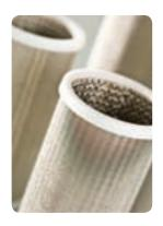
Sintered stainless steel filter elements are very useful in heavily contaminated applications and for use as pre-filters before disposable type final filters. Seals are required with these stainless steel filter elements and the options are, Viton, PTFE, or copper-alloy for high temperature applications.
